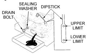
Figure 30. Draining Engine Oil
